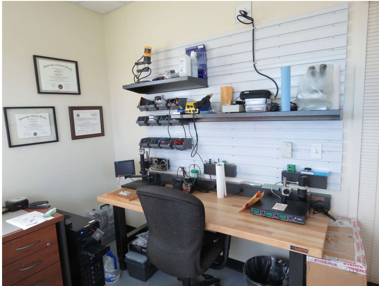
Chip-Off station for removing microchips from cell phones for further analysis
