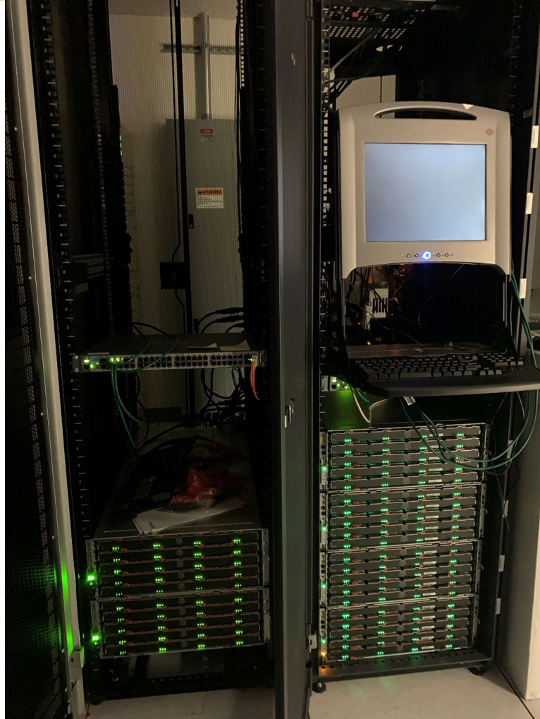
The evidence server now has 1 Petabyte of storage + a 1 Petabyte backup server.
