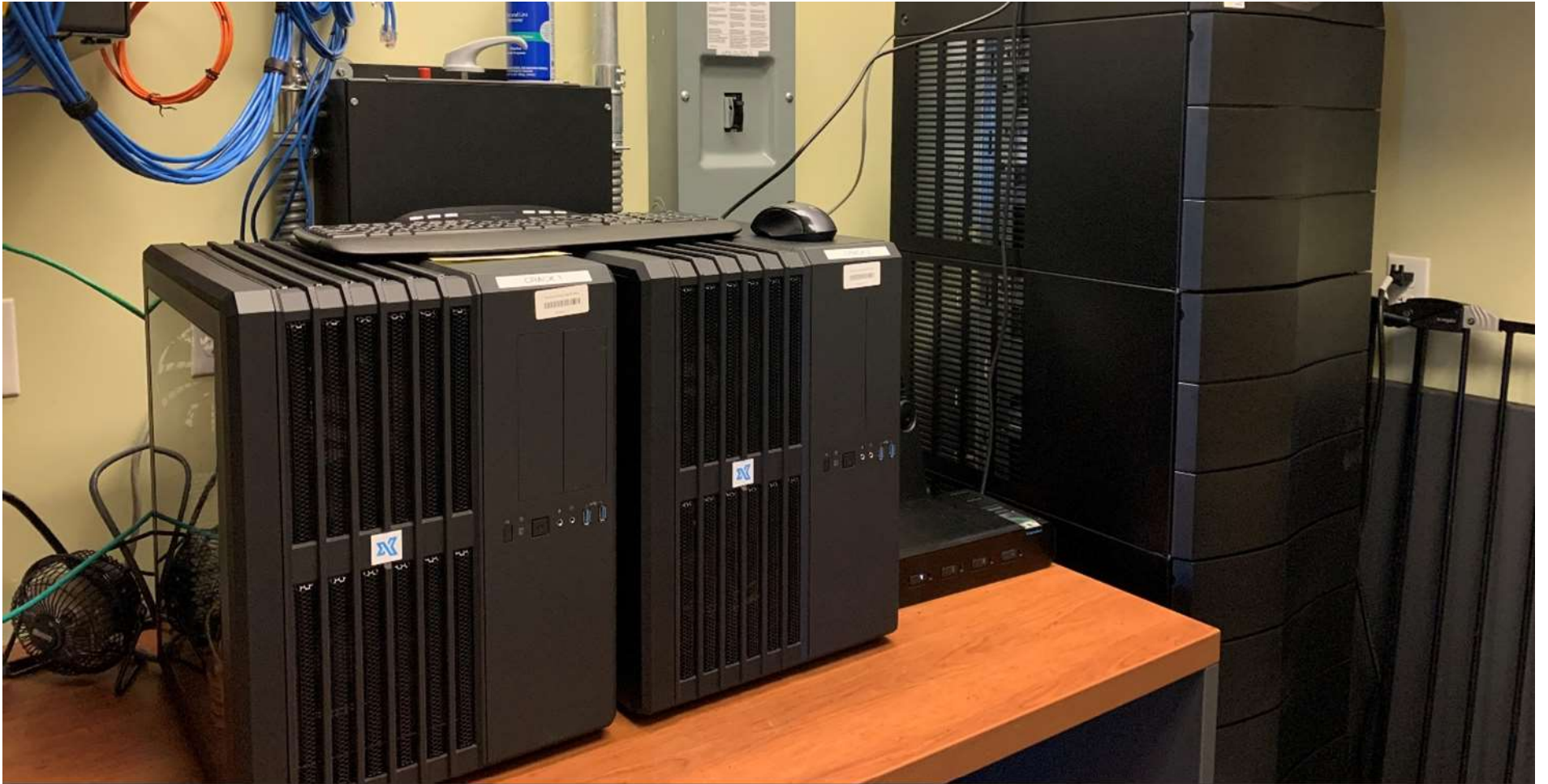
Password cracking machine built with 4 Nvidia 2080 graphic cards each
